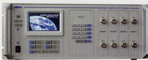
The SLE900 Satellite Link Emulator series operates at satcom intermediate frequencies (IF) and features a large touchscreen display for ease of control.
